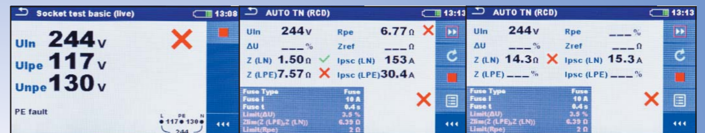
Earth Open Circuit FAIL Result
